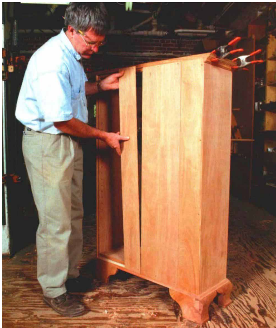
Shiplapping allows solid boards to move. A single screw placed near one edge of each board (at top and bottom) will enable each rabbeted board to hold down the board next to it, while allowing each board to move with seasonal changes.
